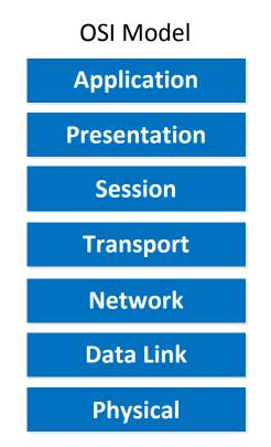
The OSI model describes a layered approach of a network, getting into the details of all the different layers of the OSI model is outside the scope of the book, but to get an **understanding of broadcasts it's important to look at layer 2 and layer 3.**
