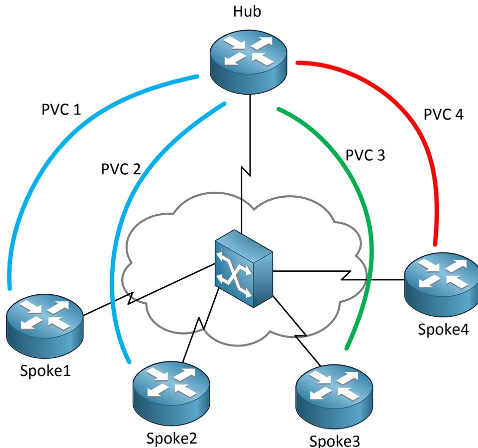
In the example above I have 5 routers in a hub and spoke model. The router on top is our hub and I have 4 spoke routers at the bottom. For each spoke there is a PVC and they each have a different CIR:
