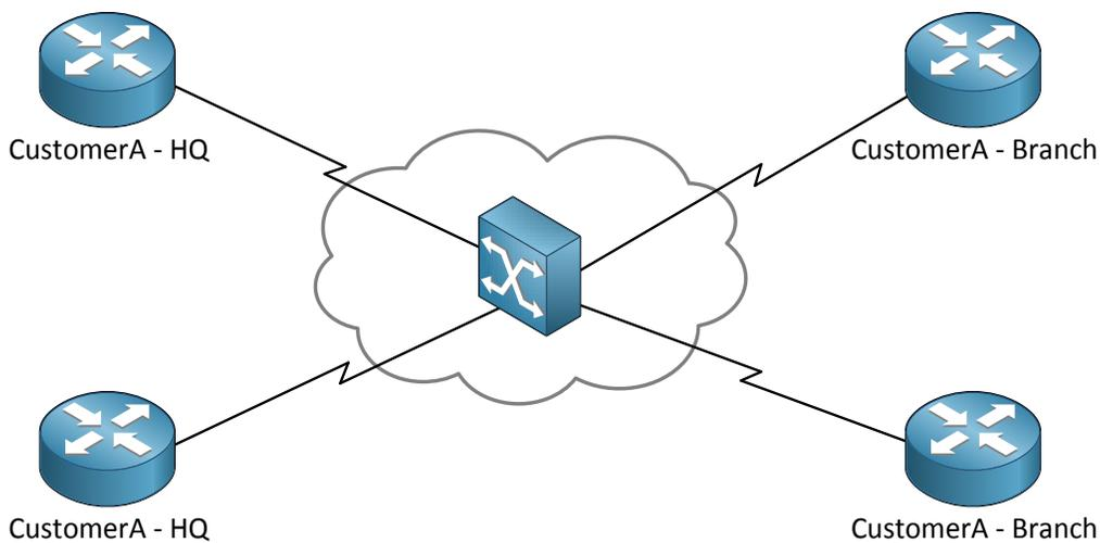
This is a picture of frame-relay. The idea behind frame-relay is that you have a single infrastructure from the service provider and multiple customers are connected to it, effectively sharing everything.
