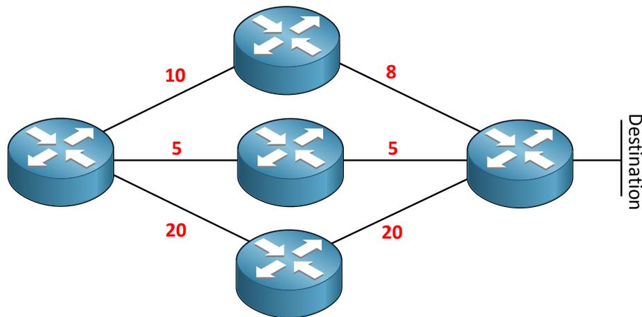
Look at the picture above, we are sitting in the router on the left and running the SPF algorithm looking for the shortest path to our destination. Which one are we going to use?
