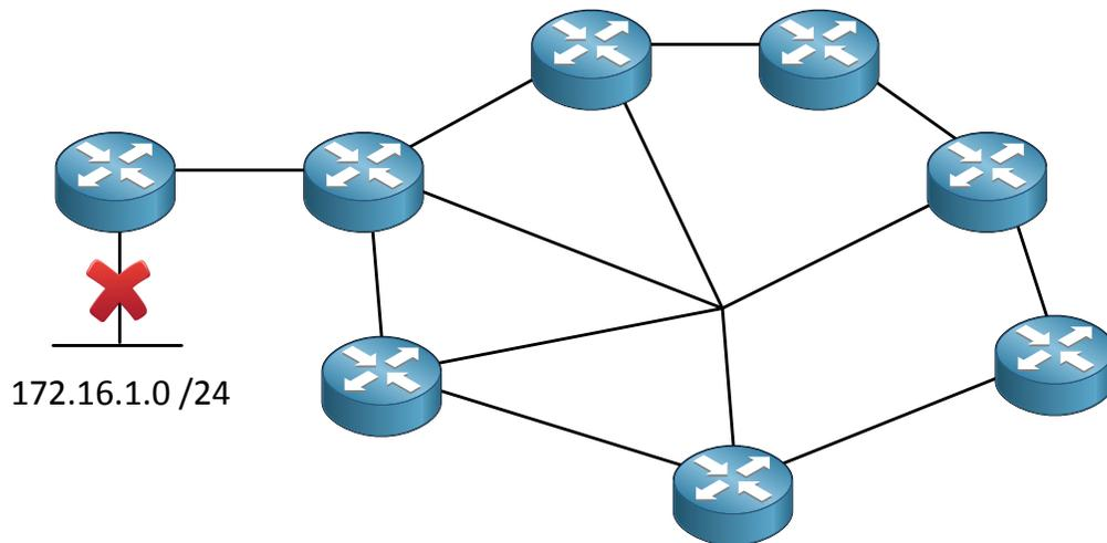
Look at the topology above. We are running EIGRP on all routers. The router on the left side has an interface that's going down.
