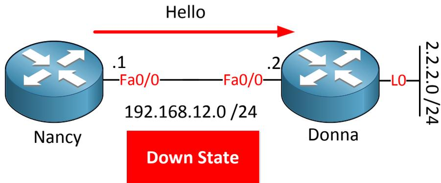
As soon as I configure OSPF on router Nancy it will start sending hello packets. Router Nancy has no clue about other OSPF routers at this moment so it's in the **down state**. The hello packet will be sent to the **multicast address 224.0.0.5**.
