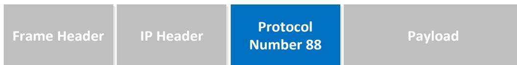
EIGRP runs directly on top of the IP header. If you look at the picture above you see we have a frame header (for example an Ethernet Frame), an IP Header (we are using IPv4) and inside the IP packet you'll find EIGRP. EIGRP has its own protocol number which is 88. Other protocol numbers you are familiar with are TCP (6) and UDP (17).
