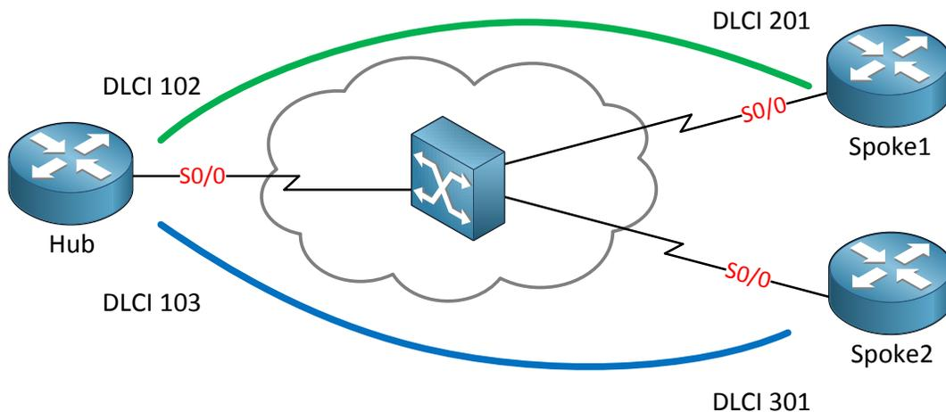
The topology above is the one I'm going to use to show you how to run EIGRP over a frame-relay network. On the left side we have a hub router and on the right side 2 spoke routers. This is a classic example of a hub and spoke model and ideal for a lab.
