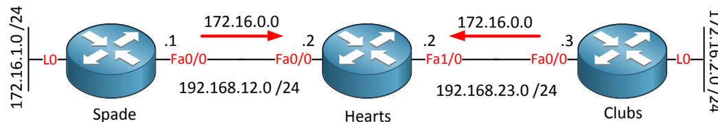
Router Spade and router Clubs don't send the subnet mask along with the routing update so it will advertise the classful network which is 172.16.0.0 in this case. So what happens with router Hearts? It thinks it can reach the 172.16.0.0 network by sending packets either left or right and if the metric is equal it will try to load-balance. Obviously this is going to cause problems.
