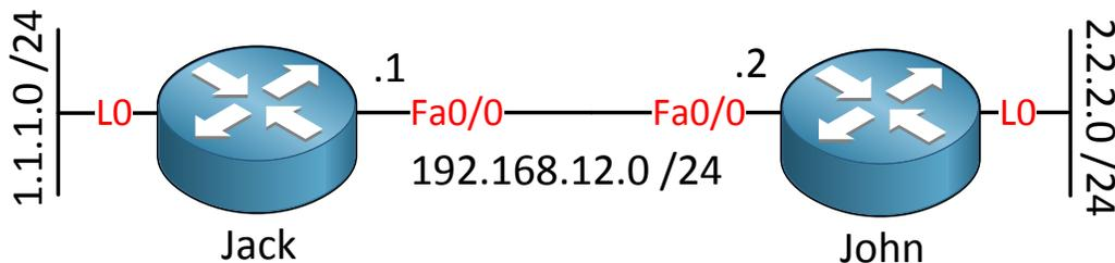
This is the topology I'm going to use to configure EIGRP. My goal is to have full connectivity and here are the configurations:
