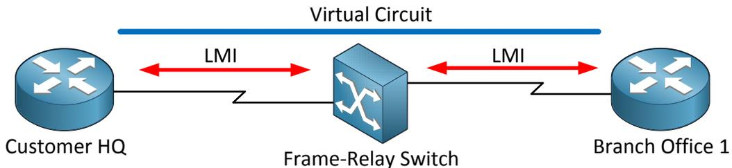
Here's an example of LMI in action. In the middle we have the frame-relay switch. LMI packets are sent between Router A and the frame-relay switch and router B and the frame-relay switch. The frame-relay switch tells our routers that the PVC is active.
