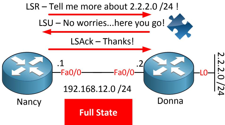
When router Nancy requested information about 2.2.2.0 /24 it used a LSR. Router Donna will send the LSU with the information. Router Nancy will send an acknowledgment using a LSAck packet to finish. We are now in the **full state**. Both routers have a synchronized LSDB and we are ready to route!
