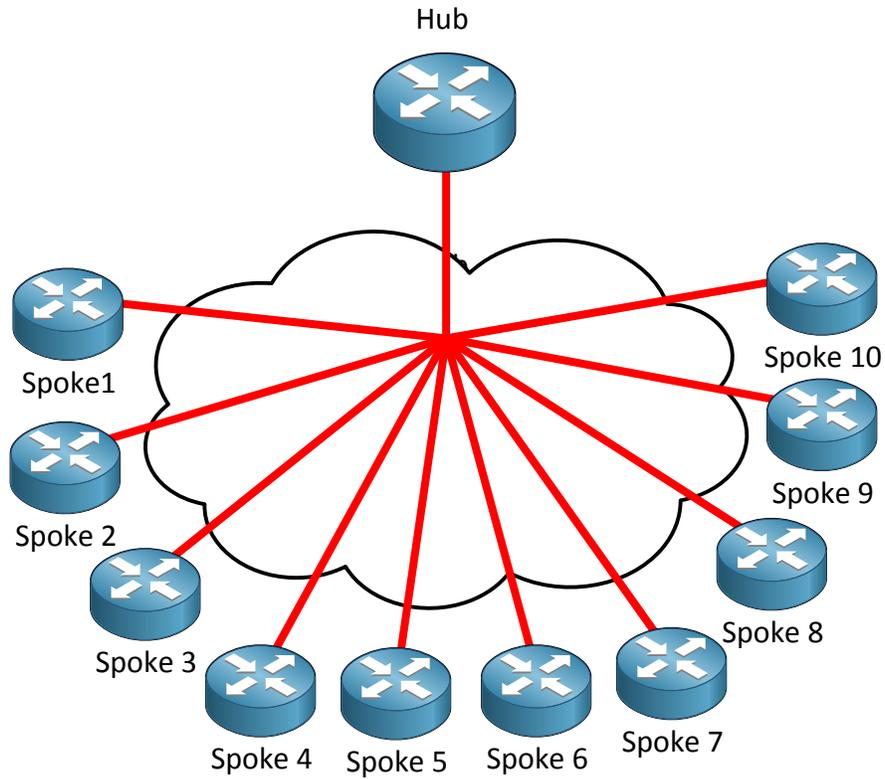
In the topology above I have one hub router and 10 spoke routers. All the PVCs are configured as point-to-point and have a CIR of 64kbps. The physical interface at the hub router only has a bandwidth of 256kbps and has been configured correctly.
