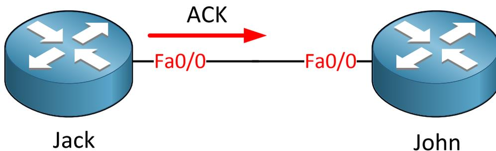
4. After both routers have exchanged hello packets we will establish the neighbor adjacency. Router Jack will send an ACK to let John know he received the update packets. The routing information in the update packets will be saved in the EIGRP topology table.
