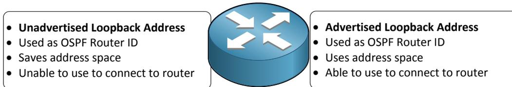
Each OSPF router needs to have a unique router ID which is based on the **highest IP address** on any **active interface**.
