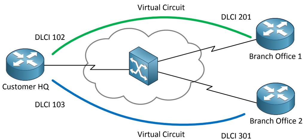
For each PVC you will get a DLCI per router. In our example above you can see that for the PVC between router HQ and branch office 1 we have DLCI 102 on the HQ router and DLCI 201 on the branch office 1 router.
