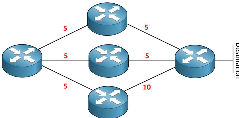
Look at this picture: As you can see the path through the router on top and the middle router have the same cost ( $5+5 = 10$ ). What are we going to do here? The path is equal.
