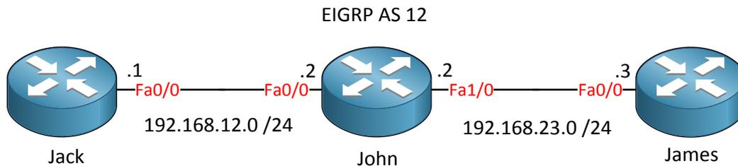
I'll use a different topology to demonstrate the different stub options. Here are the EIGRP configurations of the 3 routers:
