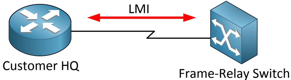
Frame-relay uses something called **LMI** which stands for **Local Management Interface**. LMI has two functions:
