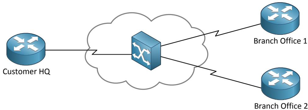
One more picture, here's a frame-relay network with three routers from one company. There's a router at the headquarters and we have two branch offices. All of them are connected to the frame-relay cloud.
