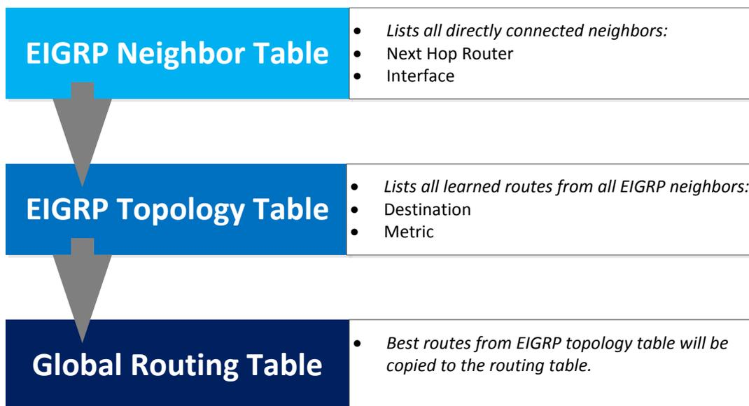
Instead of using just a single routing table EIGRP will use multiple tables. The first one is the **neighbor table** and this is where EIGRP stores all information of directly connected
