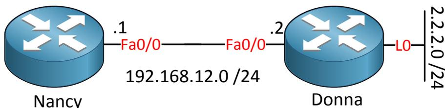
This is the topology I'm using. Router Nancy and Donna are connected using a single link
