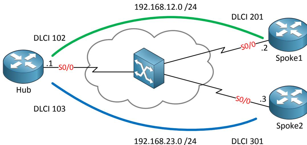
We are using the same topology to demonstrate point-to-point EIGRP over frame-relay with one difference. Point-to-point links require an **IP Subnet per PVC**:
