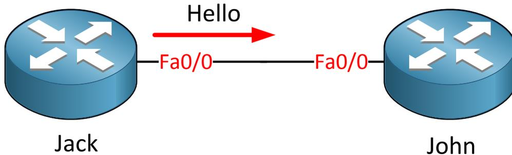
1. We have 2 routers called Jack and John and they are configured for EIGRP. As soon as we enable it for the interface they will start sending hello packets. In this example router Jack is the first router to send a hello packet.
