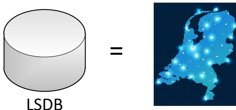
Once every router has a complete map we can start calculating the shortest path to all the different destinations by using the **shortest-path first (SPF) algorithm**. The BEST information goes into the routing table. Calculating the shortest path is like using your navigation system, it will look at the map and look at all the different ways of getting to the destination and only show you the best way of getting there.
