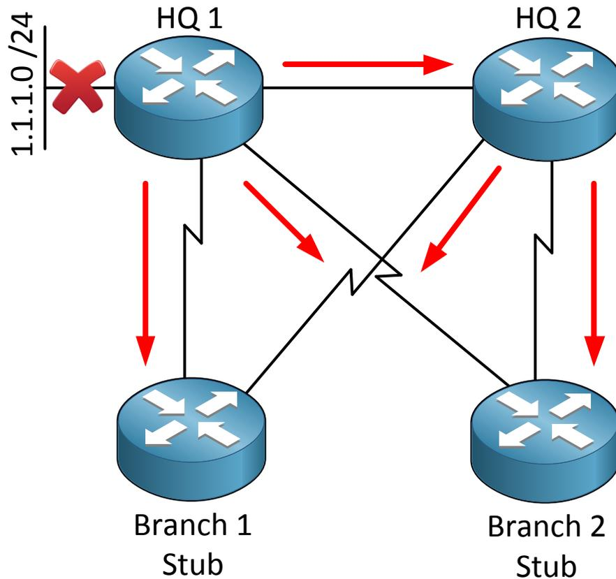
Query packets (red arrows) will fly everywhere! It doesn't sound like a good idea to use the serial links for backup so we are going to change this behavior by turning the branch routers into **EIGRP stubs**.
