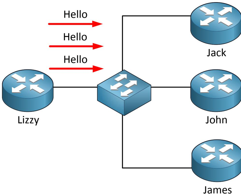
In this example we have 4 routers all running EIGRP. Hello packets are sent between routers in order to form adjacencies. As you can see router Lizzy is sending 3 hello packets meant for router Jack, John and James.
