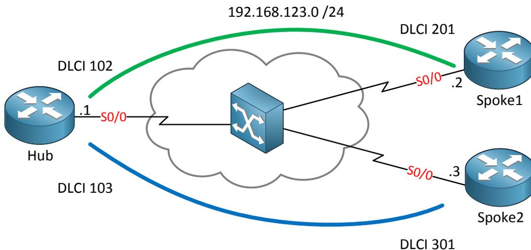
Same topology but I added the 192.168.123.0 /24 subnet. As you can see our Hub router has the .1 IP address, Spoke1 has .2 and Spoke2 has .3.
