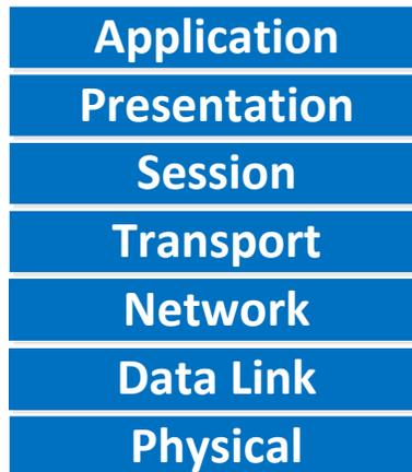
WAN protocols describe the physical (layer 1) and data link (layer 2) layer. What does frame-relay use on the data link layer? We don't use MAC addresses since that's Ethernet but we do have something else called a **DLCI (Data Link Connection Identifier)**.
